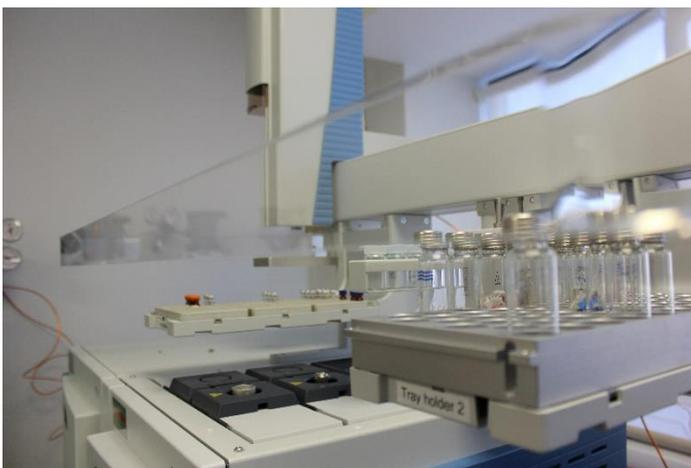
*Figure 1. Our Thermo TSQ Duo GC-MS/MS instrument is equipped with adaptors for small and large vials and an autosampler that can inject gaseous (head space), liquid or SPME fibres for concentrating volatile samples.*
